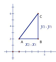
The length joining the point A and C can be found by using Pythagoras' Theorem:
